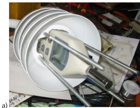
Fig. 8. Noise monitoring station: a) Design of a noise monitoring station; b) General view of the installed noise monitoring station.
