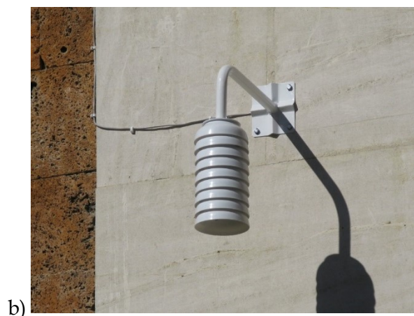
Fig. 8. Noise monitoring station: a) Design of a noise monitoring station; b) General view of the installed noise monitoring station.
