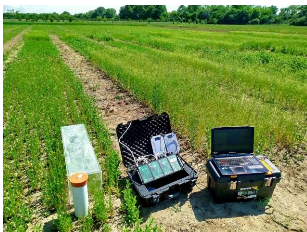
Fig. 1. Measurement of CO 2 emissions from soil (with and without vegetation) using a portable measuring device Q-box CO650, Qubit Systems Inc., Canada (May, 2024).
