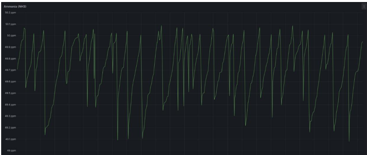
Fig. 5. Measurement data from Grafana showing ammonia concentration over a seven-day period.
